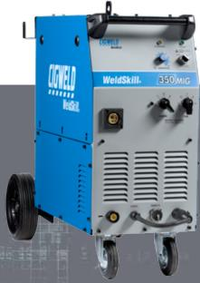
This three phase compact power source is rated at 350 amps @ 30% duty cycle and provides excellent arc performance with solid or flux cored wires. The unit is suitable for use with either mixed shielding gases, CO2 or gasless operation.
