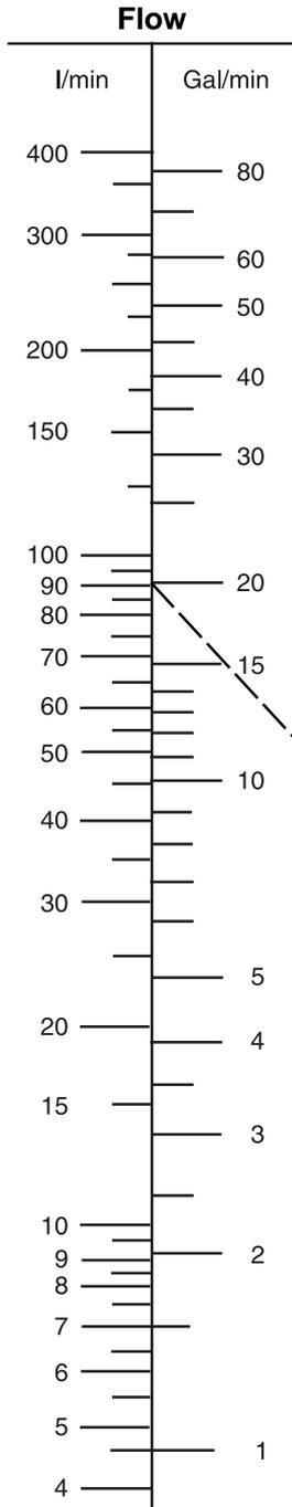
Use the chart below to determine Hose I.D. based on Flow and Velocity. Conversely, it can be used to determine Velocity, based on Flow and Hose I.D., or Flow based on Velocity and Hose I.D.
