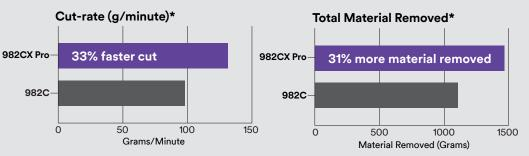
\*Results based on an automated, 11 minute test on 1018 steel using 3M<sup>™</sup> Cubitron<sup>™</sup> II Fibre Discs 982CX Pro, 7<sup>°</sup>, grade 36+ and 3M<sup>™</sup> Disc Pad Face Plate Ribbed 80514 on a servo motor.
