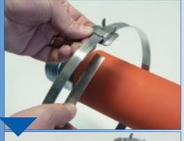
Pull buckle on band, ears pointing towards end of band. Form clamp, holding band on band, then push buckle back over the doubled band, bending the end approx. 1" under buckle.
