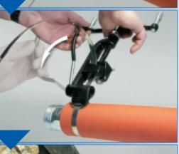
Pull on cutter lever, band is cut off to correct length.
